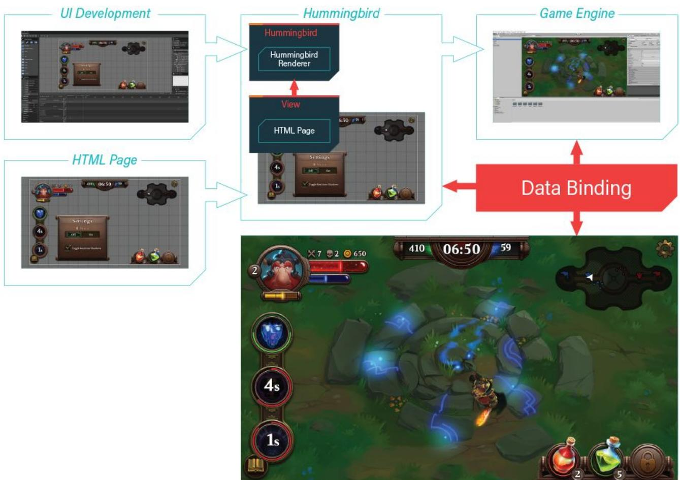
Above you can see the basic functional diagram of **Hummingbird**. Essentially, the result of the **UI development** is a HTML page that is placed inside of **Hummingbird View**. The **Hummingbird View** is a HTML5 page and the JavaScript context for it. The **View** allows you to perform various operations on the page, such as resizing, navigating to a different URL, sending input events, executing custom JavaScript code and so on. The HTML content in the **View** is rendered by the
